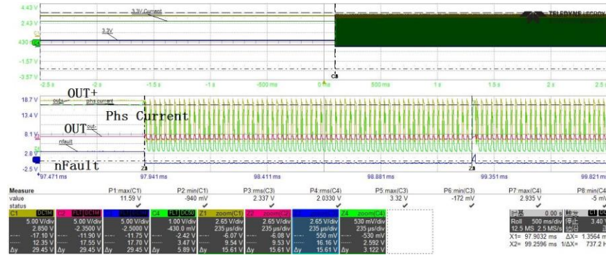
Fig. 2 Measured OUT+(C1 Yellow), OUT-(C2 Red), nFault(C3 Blue), Phs Current(C4 Green) @ bus = 12V
