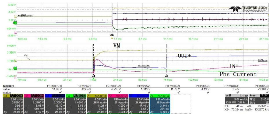
Fig. 3 Measured VM(C1 Yellow), IN+(C2 Red), OUT+(C3 Blue), Phs Current(C4 Green) @battery voltage =11.4V Power On Time =75.4us
