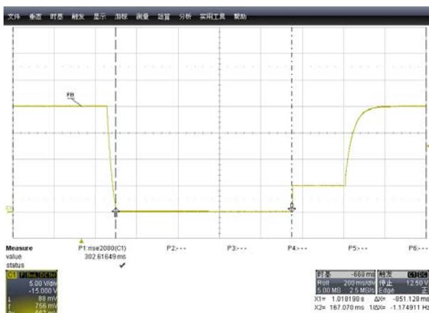
Fig. 22 Hard Reset tSrcRecover (660ms<spec<1s)
