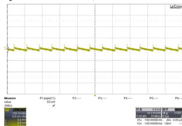
Fig. 6 Measured ripple&amp; noise waveform @90Vac/60HZ, no load.
