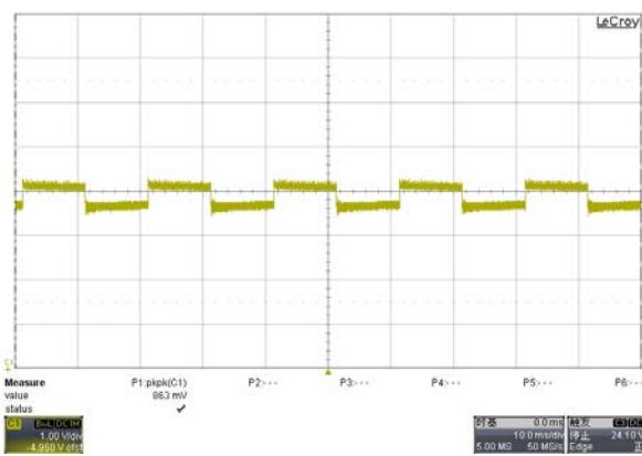
Fig. 11 Dynamic waveform @264Vac input
