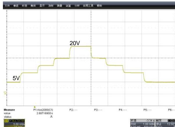
Fig. 15 Vbus Changing Test @full load
