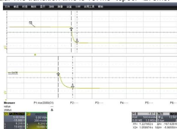
Fig. 17 Vbus Change From 20V to 5V @full load
