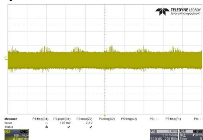
Fig. 7 Measured ripple&amp; noise waveform @90Vac/60HZ, full load.
