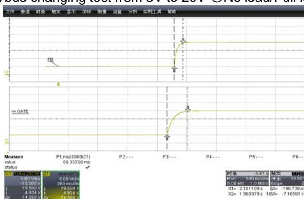
Fig. 18 Vbus Change From 5V to 20V @no load
