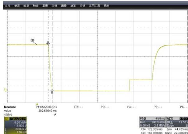
Fig. 21 Hard Reset t0-tSafe0V (spec: <650ms)
