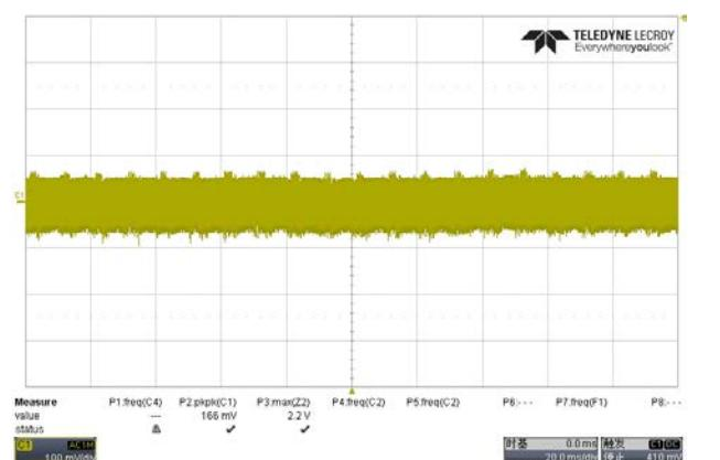
Fig. 9 R&amp;N waveform @264Vac; full load
