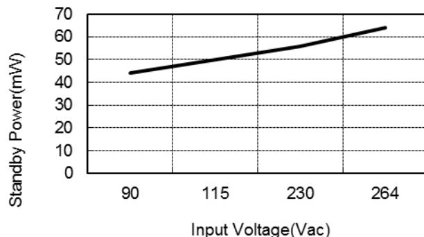
Fig. 1 No-load Input Power vs. Input Line Voltage
