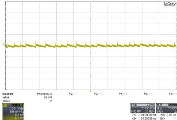
Fig. 2 Measured ripple& noise waveform@90Vac/60HZ, no load.
