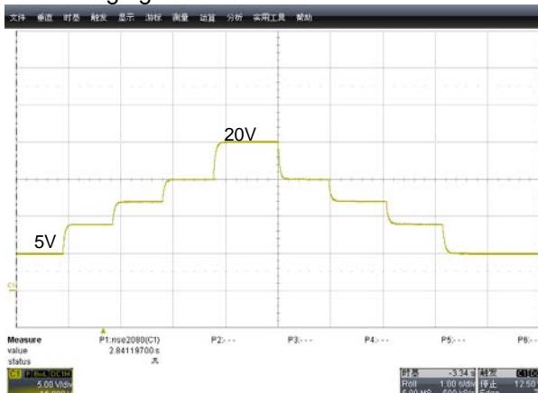
Fig. 14 Vbus Changing Test @no load
