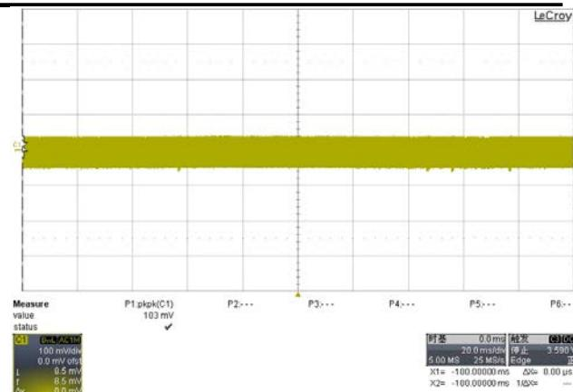
Fig. 5 R&amp;N waveform @264Vac; full load
