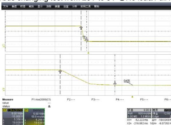
Fig. 16 Vbus Change From 20V to 5V @no load
