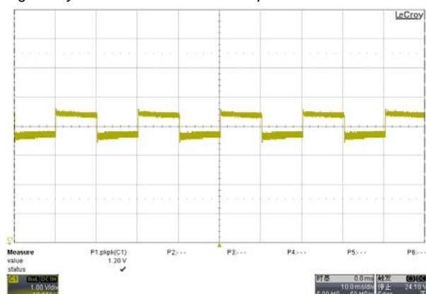
Fig. 12 Dynamic waveform @90Vac input
