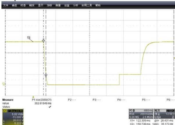
Fig. 20 Hard Reset t0-tSafe5V (spec: <275ms)
