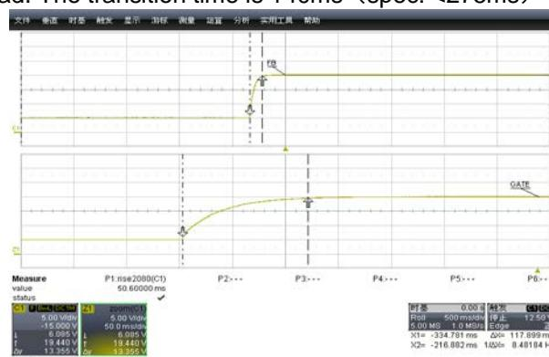
Fig. 19 Vbus Change From 5V to 20V @full load
