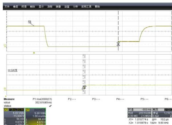
Fig. 23 Hard Reset tSrcTurnon (spec: <275ms)
