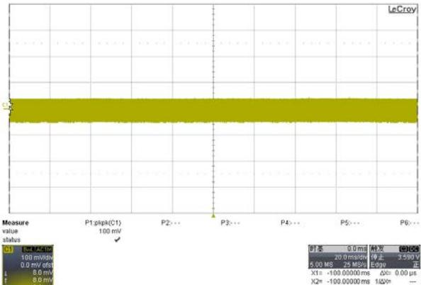
Fig. 3 Measured ripple& noise waveform@90Vac/60HZ, full load.
