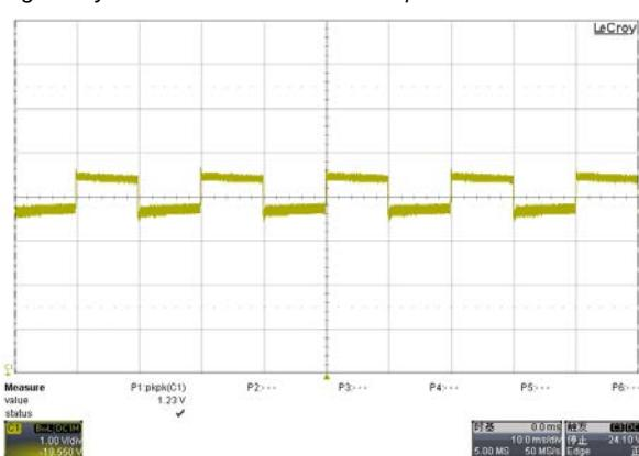
Fig. 13 Dynamic waveform @264Vac input
