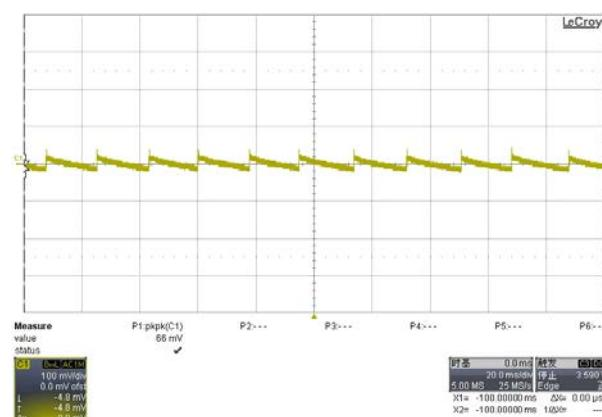
Fig. 8 R&amp;N waveform @264Vac; no load
