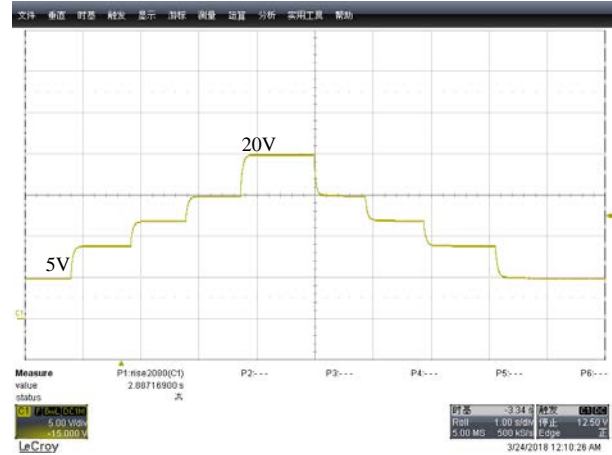
Fig. 6 Vbus Changing Test @full load
