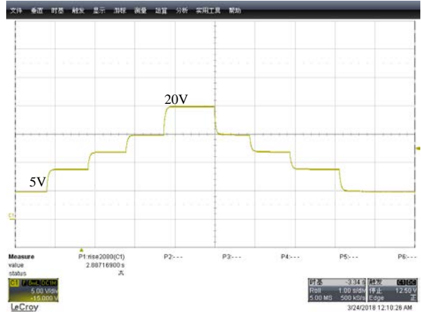
Fig. 6 Vbus Changing Test @full load
