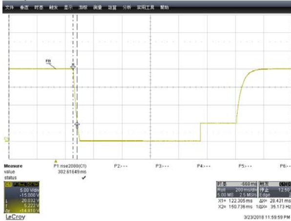
Fig. 11 Hard Reset t_{0-tSafe5V} (spec: <275ms)
