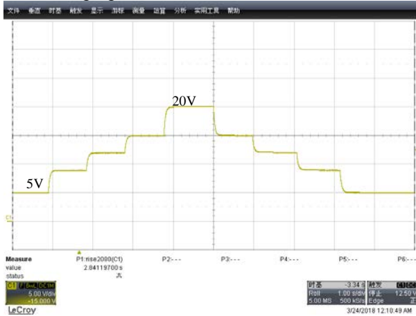
Fig. 5 Vbus Changing Test @no load
