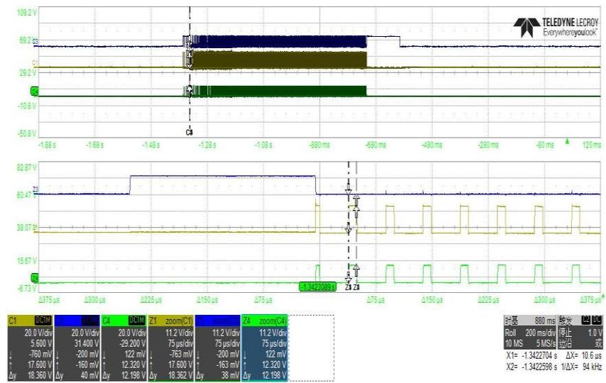
Fig. 8 Measured highside and lowside MOSFET Vgs
