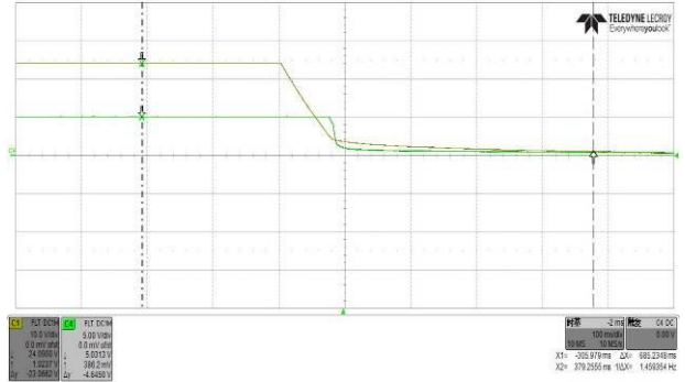
Fig. 2 Measured MCU supply voltage and DC input voltage @ input voltage =24.0V
