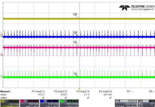
Fig. 9 CS,FB,Vdd&Vds wave form@264Vac; no load
