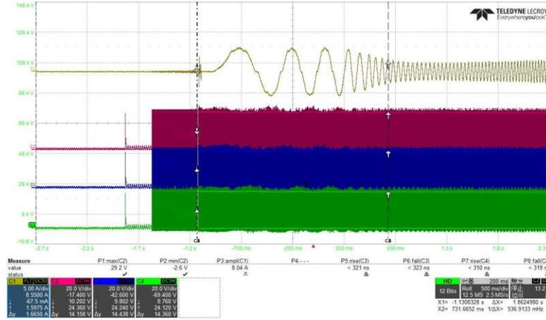
Fig. 19 Measured Phase Current(Yellow), U(Red),V(Blue),W(Green) @ Bus = 24V
