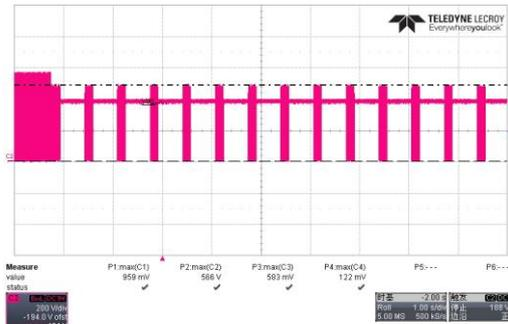
Fig. 13 Vds output short wave form @264Vac; full load
