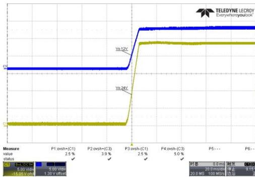
Fig. 21 Overshoot waveform @176Vac; no load
