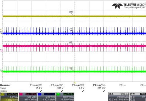
Fig. 7 CS,FB,Vdd&Vds wave form@176Vac; no load
