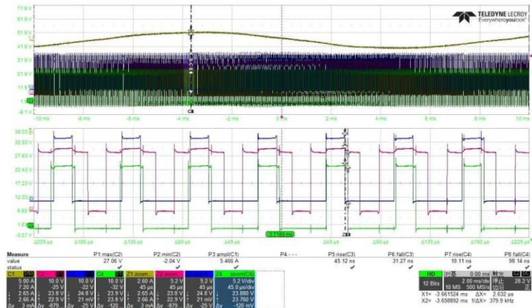
Fig. 22 Measured Phase Current(Yellow), Vds(Blue), Lowside MOS GS(Blue), Highside MOS GS(Green) @ Bus = 24V
