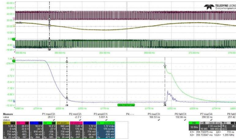
Fig. 17 Measured Phase Current(Yellow), Vds(Blue), Lowside MOS GS(Blue), Highside MOS GS(Green) @ Bus = 24V
