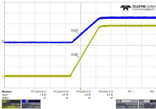
Fig. 1 Overshoot waveform @176Vac; full load
