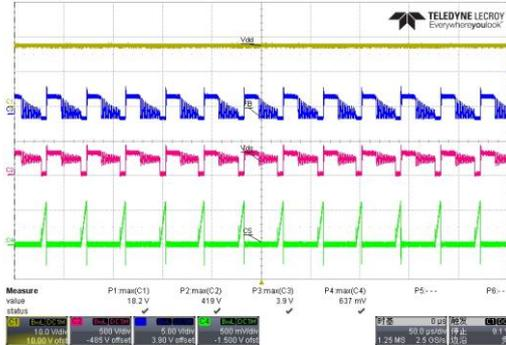
Fig. 8 CS,FB,Vdd&Vds wave form@176Vac; full load
