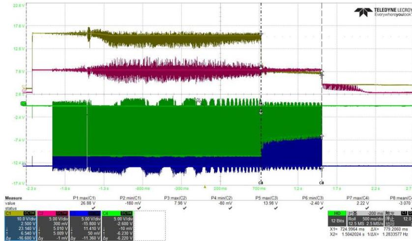
Fig. 16 Measured Bus voltage(Yellow), MCU supply voltage(Red), Lowside MOS GS(Blue), Highside MOS GS(Green) @ Bus = 24V
