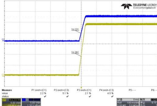
Fig. 3 Overshoot waveform @264Vac; full load
