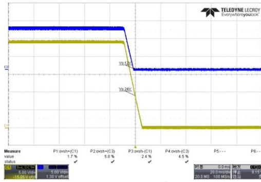
Fig. 6 Undershoot waveform @264Vac; full load
