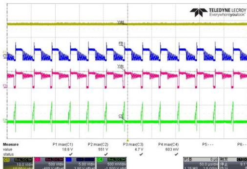
Fig. 10 CS,FB,Vdd&Vds wave form@264Vac; full load
