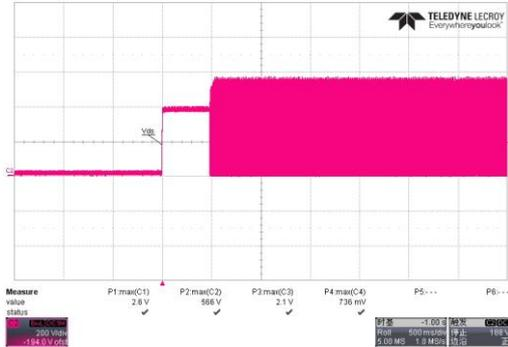
Fig. 11 Vds start up wave form @264Vac; full load
