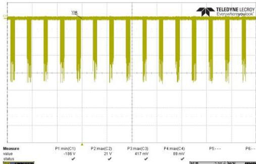
Fig. 14 Vdiode output short wave form @264Vac; full load
