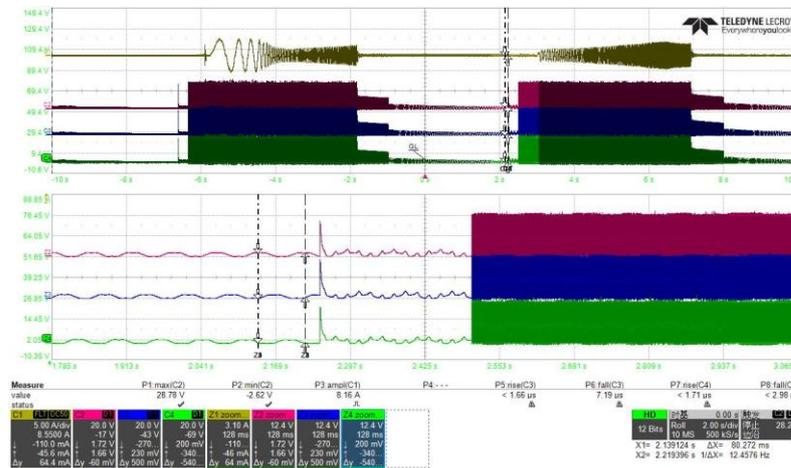
Fig. 20 Measured Phase Current(Yellow), U(Red),V(Blue),W(Green) @ Bus = 24V
