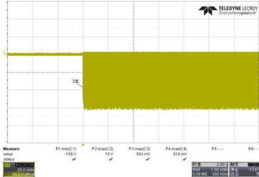
Fig. 12 Vdiode start up wave form @264Vac; full load
