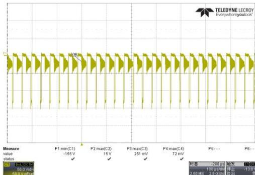
Fig. 3 Vdiode normal wave form @264Vac; full load
