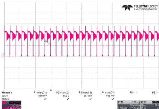
Fig. 2 Vds normal wave form @264Vac; full load
