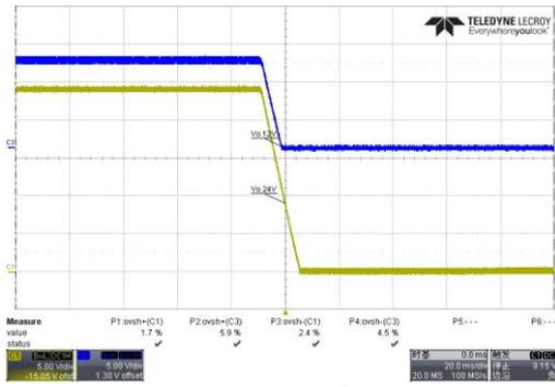
Fig. 5 Undershoot waveform@176Vac; full load
