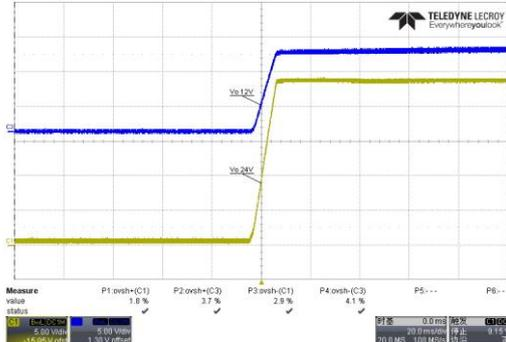
Fig. 4 Overshoot waveform @264Vac; no load
