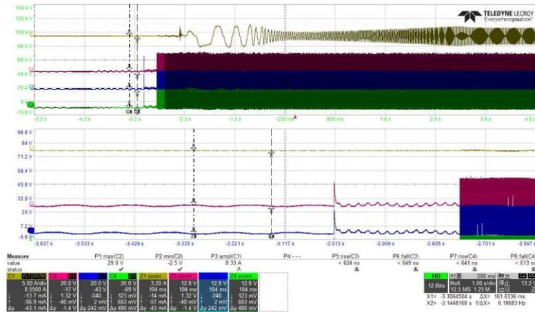
Fig. 21 Measured Phase Current(Yellow), U(Red),V(Blue),W(Green) @ Bus = 24V
