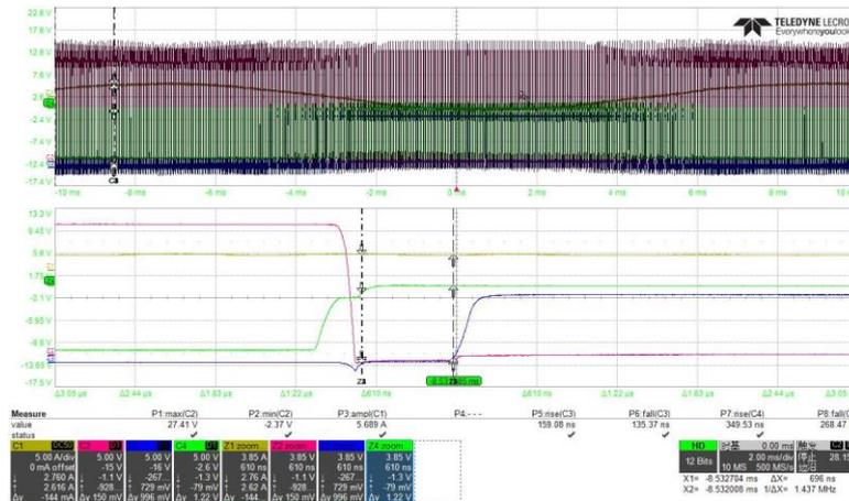
Fig. 18 Measured Phase Current(Yellow), Vds(Blue), Lowside MOS GS(Blue), Highside MOS GS(Green) @ Bus = 24V
