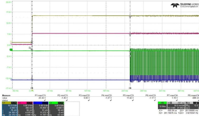
Fig. 15 Measured Bus voltage(Yellow), MCU supply voltage(Red), Lowside MOS GS(Blue), Highside MOS GS(Green) @ Bus = 24V
