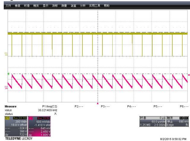
Figure 16: 264Vac, full load
