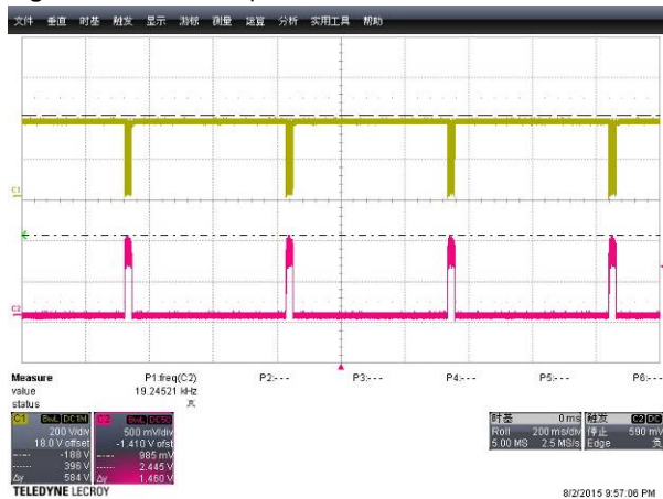
Figure 17: 264Vac, output short
