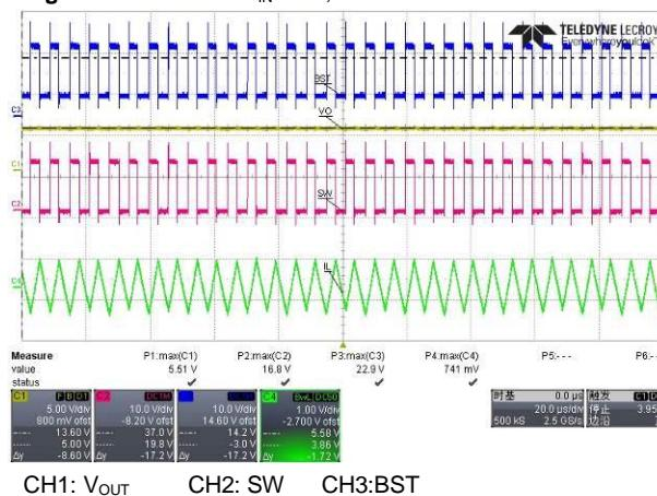
Figure 28: 5V/3.4A, V<sub>IN</sub>=12V, cc mode
