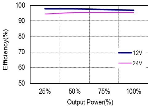
Figure 3: Efficiency @Buck CV mode VOA 9V/2.2A
