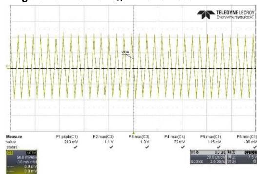
**Figure 20:** 5V/3.4A,  $V_{IN}=24V$ , full load
