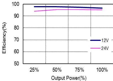
Figure 4: Efficiency @Buck CV mode VOC 9V/2.2A
