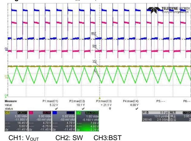
Figure 29: 5V/3.4A, V<sub>IN</sub>=12V,short
