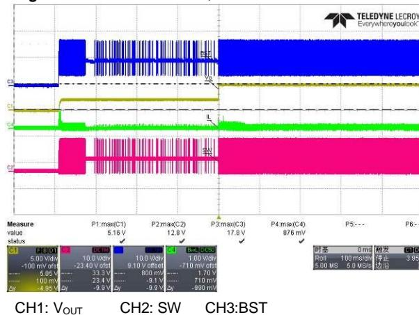
Figure 26: 5V/3.4A, V<sub>IN</sub>=12V, Normal,no load
