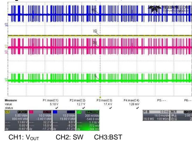
Figure 27: 5V/3.4A, V<sub>IN</sub>=12V,full load
