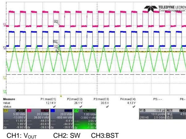
**Figure 50:** 12V/2A, V<sub>IN</sub>=24V, short
