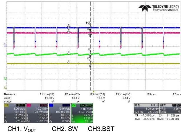
**Figure 45:** 12V/2A, V<sub>IN</sub>=12V, CC mode
