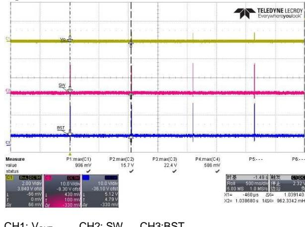
**Figure 30:** 5V/3.4A, V<sub>IN</sub>=24V, Start full load
