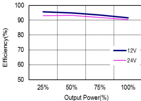
Figure 1. Efficiency @Buck CV mode VOA 5V/3.4A
