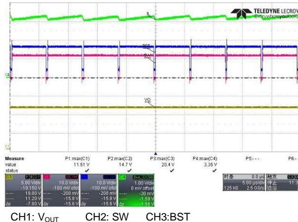
**Figure 46:** 12V/2A, V<sub>IN</sub>=12V, short
