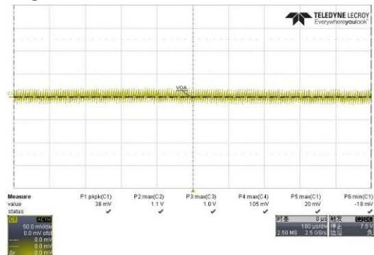
**Figure 24:** 12V/2A,  $V_{IN}=24V$ , full load
