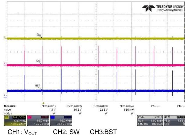
**Figure 47:** 12V/2A, V<sub>IN</sub>=24V, no load
