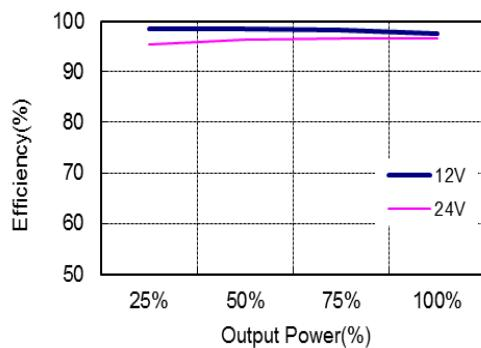
**Figure 6:** Efficiency @Buck CV mode VOC 12V/2A
