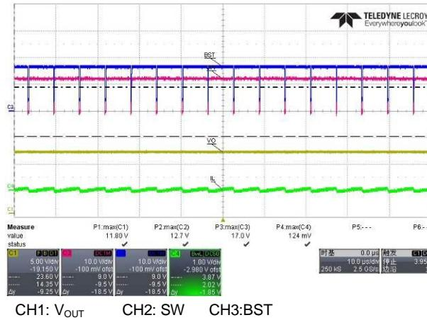
**Figure 44:** 12V/2A, V<sub>IN</sub>=12V, full load
