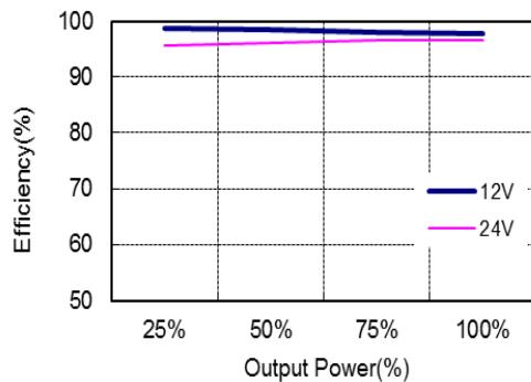
**Figure 5:** Efficiency @Buck CV mode VOA 12V/2A
