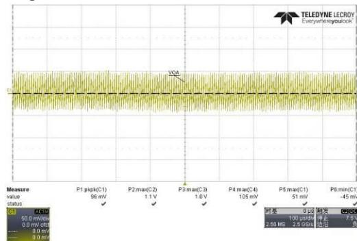
**Figure 17:** 12V/2A,  $V_{IN}=12V$ , full load
