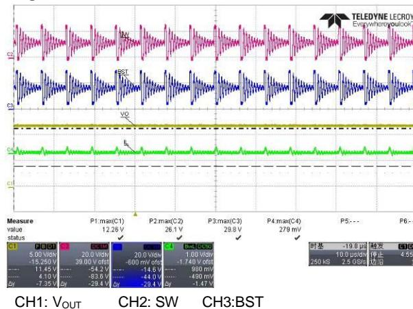
**Figure 48:** 12V/2A, V<sub>IN</sub>=24V, full load
