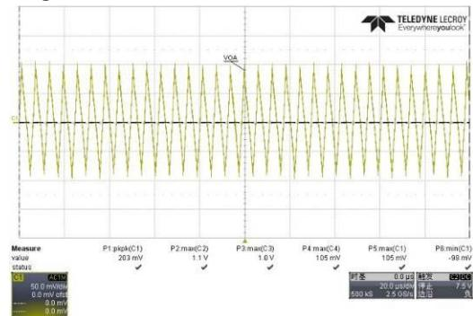
**Figure 18:** 12V/2 A,  $V_{IN}=24V$ , full load
