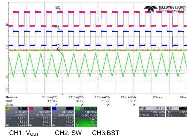
**Figure 49:** 12V/2A, V<sub>IN</sub>=24V, cc mode
